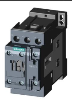
CONTACTOR, AC-3, 7.5KW/400V, 1NO+1NC, AC(40-60HZ)/DC ACTUAT. , UC 21...28V, 3-POLE, SZ SO SCREW TERMINAL
