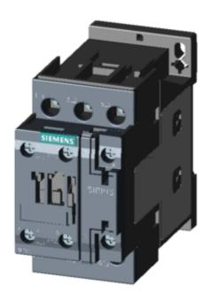
CONTACTOR, AC-3, 7.5KW/400V, 1NO+1NC, AC 400V 50HZ, 3-POLE, SZ SO SCREW TERMINAL
