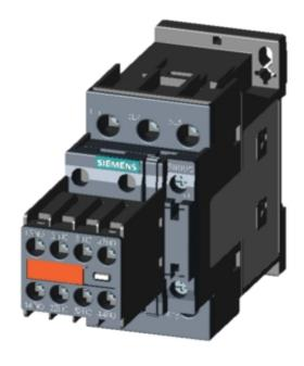
CONTACTOR, AC-3, 7.5KW/400V, 2NO+2NC, AC 230V 50/60HZ, 3-POLE, SZ SO SCREW TERMINAL PERMANENT AUX. SWITCH FOR SUVA APPLICATIONS
