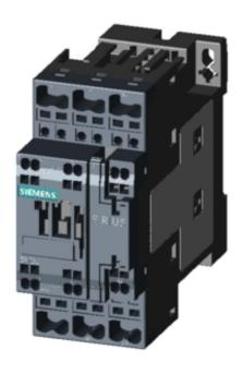
CONTACTOR, AC-3, 7.5KW/400V, 1NO+1NC, DC 24V, W.INTEGR.DIODE 3-POLE, SZ S0 SPRING-LOADED TERMINAL
