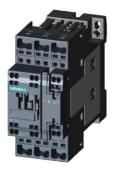
CONTACTOR, AC-3, 7.5KW/400V, 1NO+1NC, DC 110V, 3-POLE, SZ S0 SPRING-LOADED TERMINAL
