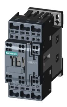
CONTACTOR, AC-3, 7.5KW/400V, 1NO+1NC, AC 230V 50HZ, 3-POLE, SZ SO SPRING-LOADED TERMINAL
