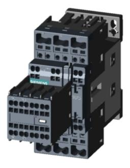
CONTACTOR, AC-3, 7.5KW/400V, 2NO+2NC, AC110V 50/60HZ, 3-POLE, SZ S0 SPRING-LOADED TERMINAL REMOVABLE AUX. SWITCH
