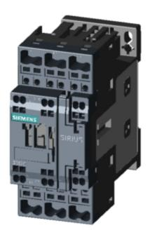
CONTACTOR, AC-3, 7.5KW/400V, 1NO+1NC, AC110V 50HZ, 120V 60HZ 3-POLE, SZ SO SPRING-LOADED TERMINAL
