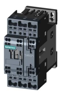
CONTACTOR, AC-3, 7.5KW/400V, 1NO+1NC, AC 24V 50HZ, 3-POLE, SZ SO SPRING-LOADED TERMINAL
