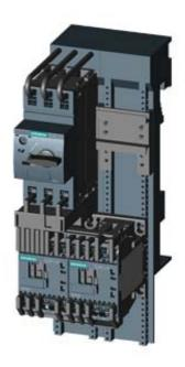
LOAD FEEDER FUSELESS REVERSING DUTY, AC 400V, SZ S00, 11. . .16A, DC 24V SPRING-LOADED CONNECTION FOR BUSBAR SYSTEMS 60MM TYPE OF COORDINATION 1, IQ = 150KA 1NC (CONTACTOR)
