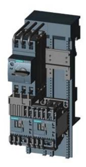
LOAD FEEDER FUSELESS REVERSING DUTY, AC 400V, SZ S00, 5,5. . .8A, AC 230V SPRING-LOADED CONNECTION FOR BUSBAR SYSTEMS 60MM TYPE OF COORDINATION 1, IQ = 150KA 1NC (CONTACTOR)
