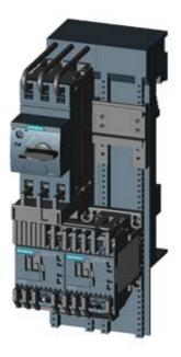
LOAD FEEDER FUSELESS REVERSING DUTY, AC 400V, SZ S00, 4.5. . .6.3A, DC 24V SPRING-LOADED CONNECTION FOR BUSBAR SYSTEMS 60MM TYPE OF COORDINATION 1, IQ = 150KA 1NC (CONTACTOR)
