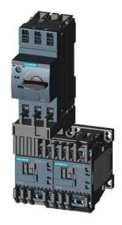
LOAD FEEDER FUSELESS REVERSING DUTY, AC 400V, SZ S00, 4.5. . . 6.3A, DC 24V SPRING-LOADED CONNECTION FOR RAIL-MOUNTING, TYPE OF COORDINATION 1, IQ = 150KA 1NC (CONTACTOR)
