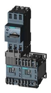
LOAD FEEDER FUSELESS REVERSING DUTY, AC 400V, SZ S00, 4.5...6.3A, AC 230V SPRING-LOADED CONNECTION FOR RAIL-MOUNTING, TYPE OF COORDINATION 1, IQ = 150KA 1NC (CONTACTOR)
