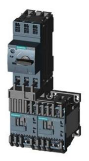
LOAD FEEDER FUSELESS REVERSING DUTY, AC 400V, SZ S00, 3.5. . .5A, DC 24V SPRING-LOADED CONNECTION FOR RAIL-MOUNTING, TYPE OF COORDINATION 1, IQ = 150KA 1NC (CONTACTOR)
