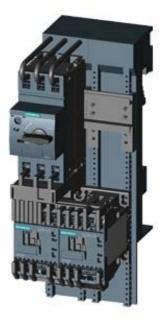
LOAD FEEDER FUSELESS REVERSING DUTY, AC 400V, SZ S00, 1.8. . .2.5A, DC 24V SPRING-LOADED CONNECTION FOR BUSBAR SYSTEMS 60MM TYPE OF COORDINATION 2, IQ = 150KA (ALSO FULFILLS TYPE OF COORDINATION 1) 1NC (CONTACTOR)
