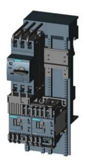
LOAD FEEDER FUSELESS REVERSING DUTY, AC 400V, SZ S00, 1.1...1.6A, AC 230V SPRING-LOADED CONNECTION FOR BUSBAR SYSTEMS 60MM TYPE OF COORDINATION 2, IQ = 150KA (ALSO FULFILLS TYPE OF COORDINATION 1) 1NC (CONTACTOR)
