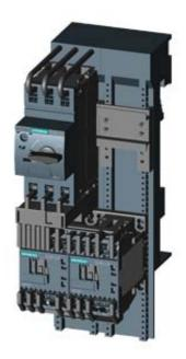
LOAD FEEDER FUSELESS REVERSING DUTY, AC 400V, SZ S00, 1.4. . .2A, AC 230V SPRING-LOADED CONNECTION FOR BUSBAR SYSTEMS 60MM TYPE OF COORDINATION 2, IQ = 150KA (ALSO FULFILLS TYPE OF COORDINATION 1) 1NC (CONTACTOR)
