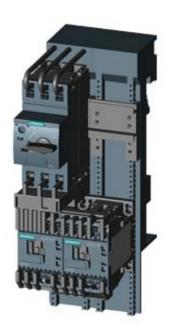
LOAD FEEDER FUSELESS REVERSING DUTY, AC 400V, SZ S00, 0.28...0.4A, AC 230V SPRING-LOADED CONNECTION FOR BUSBAR SYSTEMS 60MM TYPE OF COORDINATION 2, IQ = 150KA (ALSO FULFILLS TYPE OF COORDINATION 1) 1NC (CONTACTOR)
