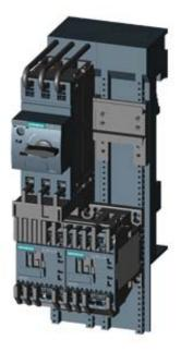
LOAD FEEDER FUSELESS REVERSING DUTY, AC 400V, SZ S00, 0.22...0.32A, AC 230V SPRING-LOADED CONNECTION FOR BUSBAR SYSTEMS 60MM TYPE OF COORDINATION 2, IQ = 150KA (ALSO FULFILLS TYPE OF COORDINATION 1) 1NC (CONTACTOR)
