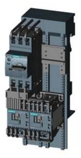
LOAD FEEDER FUSELESS REVERSING DUTY, AC 400V, SZ S00, 0.14...0.2A, AC 230V SPRING-LOADED CONNECTION FOR BUSBAR SYSTEMS 60MM TYPE OF COORDINATION 2, IQ = 150KA (ALSO FULFILLS TYPE OF COORDINATION 1) 1NC (CONTACTOR)
