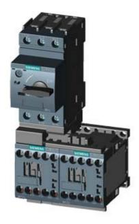
LOAD FEEDER FUSELESS REVERSING DUTY, AC 400V, SZ S00, 11...16A, AC 230V SCREW CONNECTION FOR RAIL-MOUNTING, TYPE OF COORDINATION 1, IQ = 150KA 1NC (CONTACTOR)
