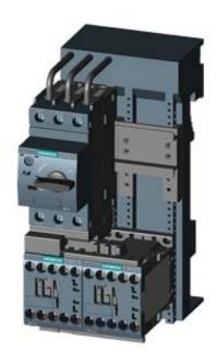
LOAD FEEDER FUSELESS REVERSING DUTY, AC 400V, SZ S00, 7...10A, AC 230V SCREW CONNECTION FOR BUSBAR SYSTEMS 60MM TYPE OF COORDINATION 1, IQ = 150KA 1NC (CONTACTOR)
