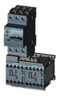
LOAD FEEDER FUSELESS REVERSING DUTY, AC 400V, SZ S00, 9. . . 12.5A, AC 230V SCREW CONNECTION FOR RAIL-MOUNTING, TYPE OF COORDINATION 1, IQ = 150KA 1NC (CONTACTOR)
