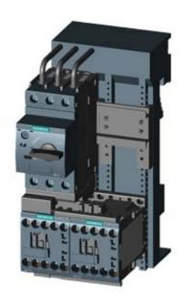
LOAD FEEDER FUSELESS REVERSING DUTY, AC 400V, SZ S00, 3.5. . .5A, DC 24V SCREW CONNECTION FOR BUSBAR SYSTEMS 60MM TYPE OF COORDINATION 1, IQ = 150KA 1NC (CONTACTOR)
