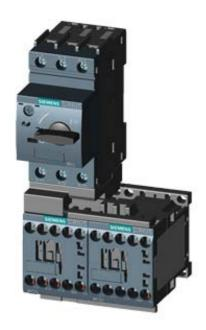
LOAD FEEDER FUSELESS REVERSING DUTY, AC 400V, SZ S00, 3.5. . .5A, AC 230V SCREW CONNECTION FOR RAIL-MOUNTING, TYPE OF COORDINATION 1, IQ = 150KA 1NC (CONTACTOR)
