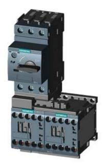
LOAD FEEDER FUSELESS REVERSING DUTY, AC 400V, SZ S00, 2.8. . .4A, AC 230V SCREW CONNECTION FOR RAIL-MOUNTING, TYPE OF COORDINATION 2, IQ = 150KA (ALSO FULFILLS TYPE OF COORDINATION 1) 1NC (CONTACTOR)
