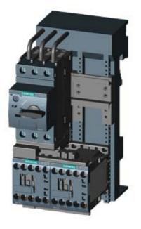
LOAD FEEDER FUSELESS REVERSING DUTY, AC 400V, SZ S00, 1.8. . .2.5A, AC 230V SCREW CONNECTION FOR BUSBAR SYSTEMS 60MM TYPE OF COORDINATION 2, IO = 150KA (ALSO FULLEULS TYPE OF COORDINATION 1)
