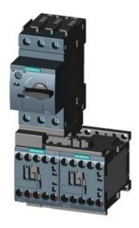
LOAD FEEDER FUSELESS REVERSING DUTY, AC 400V, SZ S00, 1.4. . .2A, AC 230V SCREW CONNECTION FOR RAIL-MOUNTING, TYPE OF COORDINATION 2, IQ = 150KA (ALSO FULFILLS TYPE OF COORDINATION 1) 1NC (CONTACTOR)
