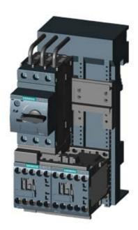
LOAD FEEDER FUSELESS REVERSING DUTY, AC 400V, SZ S00, 0.7...1A, AC 230V SCREW CONNECTION FOR BUSBAR SYSTEMS 60MM TYPE OF COORDINATION 2, IQ = 150KA (ALSO FULFILLS TYPE OF COORDINATION 1) 1NC (CONTACTOR)
