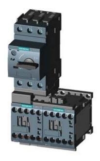
LOAD FEEDER FUSELESS REVERSING DUTY, AC 400V, SZ S00, 0.55...0.8A, AC 230V SCREW CONNECTION FOR RAIL-MOUNTING, TYPE OF COORDINATION 2, IQ = 150KA (ALSO FULFILLS TYPE OF COORDINATION 1) 1NC (CONTACTOR)
