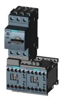
LOAD FEEDER FUSELESS REVERSING DUTY, AC 400V, SZ S00, 0.45...0.63A, DC 24V SCREW CONNECTION FOR RAIL-MOUNTING, TYPE OF COORDINATION 2, IQ = 150KA (ALSO FULFILLS TYPE OF COORDINATION 1) 1NC (CONTACTOR)
