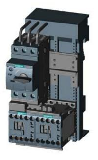
LOAD FEEDER FUSELESS REVERSING DUTY, AC 400V, SZ S00, 0.35. . .0.5A, DC 24V SCREW CONNECTION FOR BUSBAR SYSTEMS 60MM TYPE OF COORDINATION 2, IQ = 150KA (ALSO FULFILLS TYPE OF COORDINATION 1) 1NC (CONTACTOR)
