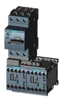
LOAD FEEDER FUSELESS REVERSING DUTY, AC 400V, SZ S00, 0.35. . .0.5A, DC 24V SCREW CONNECTION FOR RAIL-MOUNTING, TYPE OF COORDINATION 2, IQ = 150KA (ALSO FULFILLS TYPE OF COORDINATION 1) 1NC (CONTACTOR)
