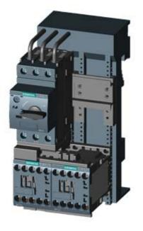
LOAD FEEDER FUSELESS REVERSING DUTY, AC 400V, SZ S00, 0.28. . .0.4A, DC 24V SCREW CONNECTION FOR BUSBAR SYSTEMS 60MM TYPE OF COORDINATION 2, IQ = 150KA (ALSO FULFILLS TYPE OF COORDINATION 1) 1NC (CONTACTOR)
