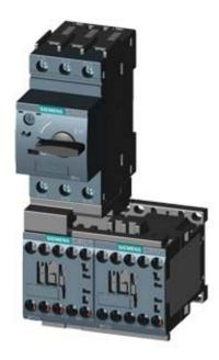
LOAD FEEDER FUSELESS REVERSING DUTY, AC 400V, SZ S00, 0.22...0.32A, AC 230V SCREW CONNECTION FOR RAIL-MOUNTING, TYPE OF COORDINATION 2, IQ = 150KA (ALSO FULFILLS TYPE OF COORDINATION 1) 1NC (CONTACTOR)
