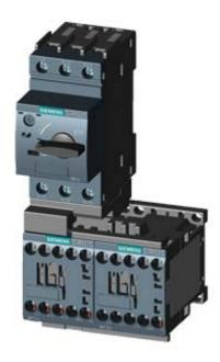
LOAD FEEDER FUSELESS REVERSING DUTY, AC 400V, SZ S00, 0.28...0.4A, AC 230V SCREW CONNECTION FOR RAIL-MOUNTING, TYPE OF COORDINATION 2, IQ = 150KA (ALSO FULFILLS TYPE OF COORDINATION 1) 1NC (CONTACTOR)
