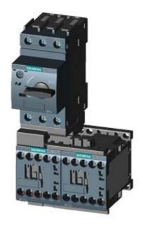
LOAD FEEDER FUSELESS REVERSING DUTY, AC 400V, SZ S00, 0.14...0.2A, AC 230V SCREW CONNECTION FOR RAIL-MOUNTING, TYPE OF COORDINATION 2, IQ = 150KA (ALSO FULFILLS TYPE OF COORDINATION 1) 1NC (CONTACTOR)
