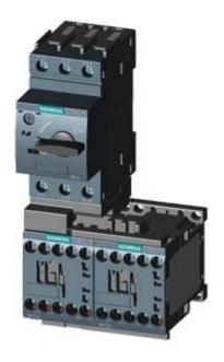
LOAD FEEDER FUSELESS REVERSING DUTY, AC 400V, SZ S00, 0.18...0.25A, AC 230V SCREW CONNECTION FOR RAIL-MOUNTING, TYPE OF COORDINATION 2, IQ = 150KA (ALSO FULFILLS TYPE OF COORDINATION 1) 1NC (CONTACTOR)
