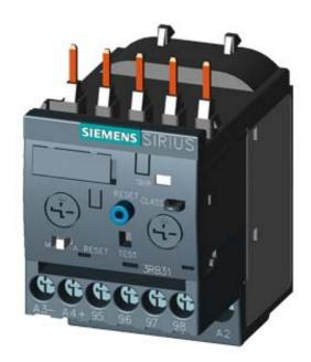
OVERLOAD RELAY 0.1...0.4 A FOR MOTOR PROTECTION SIZE S00, CLASS 5...30 CONTACTOR ASS. MAIN CIRCUIT: SCREW CONN. AUX.CIRCUIT: SCREW CONN. MANUAL-AUTOM.-RESET INT. GROUND FAULT DETECTION
