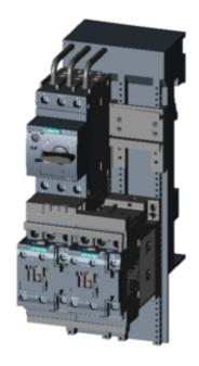
LOAD FEEDER FUSELESS REVERSING DUTY, AC 400V, SZ. S0, 27...32A, DC 24V SCREW CONNECTION FOR BUSBAR SYSTEMS 60MM TYPE OF COORD. 2,IQ = 150KA (ALSO ACHIEVES TYPE OF COORD.1) 1NO+1NC (CONTACTOR)
