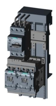
LOAD FEEDER FUSELESS REVERSING DUTY, AC 400V, SZ S0, 20. . .25A, DC 24V SCREW CONNECTION FOR BUSBAR SYSTEMS 60MM TYPE OF COORDINATION 2, IQ = 150KA (ALSO FULFILLS TYPE OF COORDINATION 1) 1NO+1NC (CONTACTOR)
