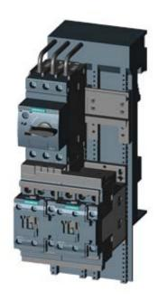
LOAD FEEDER FUSELESS REVERSING DUTY, AC 400V, SZ. S0, 9. . . 12.5A, AC 230V SCREW CONNECTION FOR BUSBAR SYSTEMS 60MM TYPE OF COORD. 2,IQ = 150KA (ALSO ACHIEVES TYPE OF COORD.1) 1NO+1NC (CONTACTOR)
