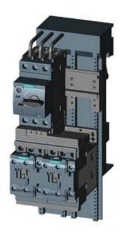
LOAD FEEDER FUSELESS REVERSING DUTY, AC 400V, SZ S0, 11...16A, AC 230V SCREW CONNECTION FOR BUSBAR SYSTEMS 60MM TYPE OF COORDINATION 2, IQ = 150KA (ALSO FULFILLS TYPE OF COORDINATION 1) 1NO+1NC (CONTACTOR)
