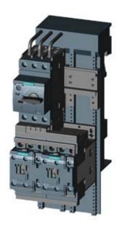
LOAD FEEDER FUSELESS REVERSING DUTY, AC 400V, SZ. S0, 7. . . 10A, AC 230V SCREW CONNECTION FOR BUSBAR SYSTEMS 60MM TYPE OF COORD. 2,IQ = 150KA (ALSO ACHIEVES TYPE OF COORD.1) 1NO+1NC (CONTACTOR)
