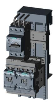
LOAD FEEDER FUSELESS REVERSING DUTY, AC 400V, SZ S0, 5,5...8A, DC 24V SCREW CONNECTION FOR BUSBAR SYSTEMS 60MM TYPE OF COORDINATION 2, IQ = 150KA (ALSO FULFILLS TYPE OF COORDINATION 1) 1NO+1NC (CONTACTOR)
