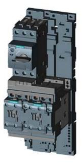
LOAD FEEDER FUSELESS REVERSING DUTY, AC 400V, SZ S0, 5,5. . .8A, DC 24V SCREW CONNECTION FOR RAIL-MOUNTING, W. DIN RAIL ADAPTER TYPE OF COORDINATION 2, IQ = 150KA (ALSO FULFILLS TYPE OF COORDINATION 1) 1NO+1NC (CONTACTOR)
