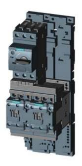
LOAD FEEDER FUSELESS REVERSING DUTY, AC 400V, SZ S0, 5,5...8A, AC 230V SCREW CONNECTION FOR RAIL-MOUNTING, W. DIN RAIL ADAPTER TYPE OF COORDINATION 2, IQ = 150KA (ALSO FULFILLS TYPE OF COORDINATION 1) 1NO+1NC (CONTACTOR)
