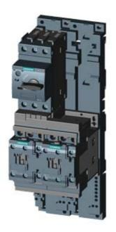
LOAD FEEDER FUSELESS REVERSING DUTY, AC 400V, SZ. S0, 7...10A, AC 230V SCREW CONNECTION FOR RAIL MOUNTING, W. MOUNTING RAIL ADAPTER TYPE OF COORD. 2,IQ = 150KA (ALSO ACHIEVES TYPE OF COORD.1) 1NO+1NC (CONTACTOR)
