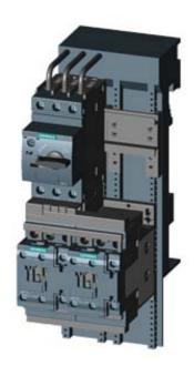
LOAD FEEDER FUSELESS REVERSING DUTY, AC 400V, SZ S0, 3.5...5A, AC 230V SCREW CONNECTION FOR BUSBAR SYSTEMS 60MM TYPE OF COORDINATION 2, IQ = 150KA (ALSO FULFILLS TYPE OF COORDINATION 1) 1NO+1NC (CONTACTOR)
